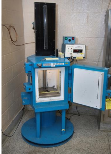
Figure 10. Photograph of J.L. Shepherd Mark I Model 68A Cesium 137 Irradiator at the Brookhaven National Laboratory used in the 662 keV gamma radiation test for the InGaAs Quad Photoreceivers (Source: www.bnl.gov/nsrl/grsf ).
