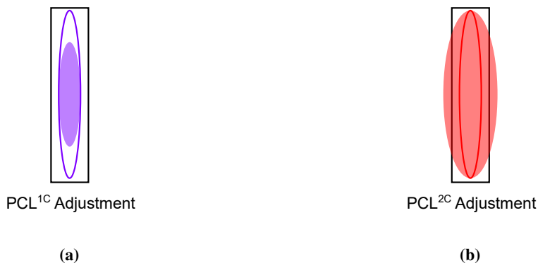
Fig. 2 Effect of adjustment of the focal length or position of (a) PCL^{1C} or (b) PCL^{2C} on the beam size incident on PD (compare colored solid outline and colored filled shape).
