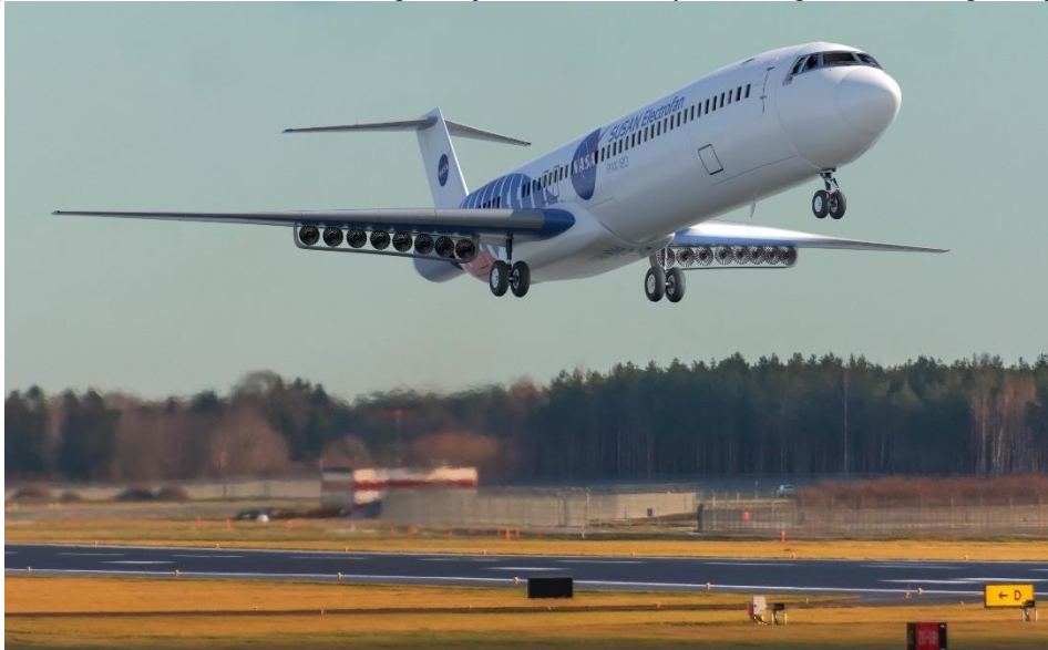
Figure 1 Artist Rendering of Subsonic Single Aft Engine (SUSAN) Transport Aircraft Concept (credit Eric S. Mindek.
