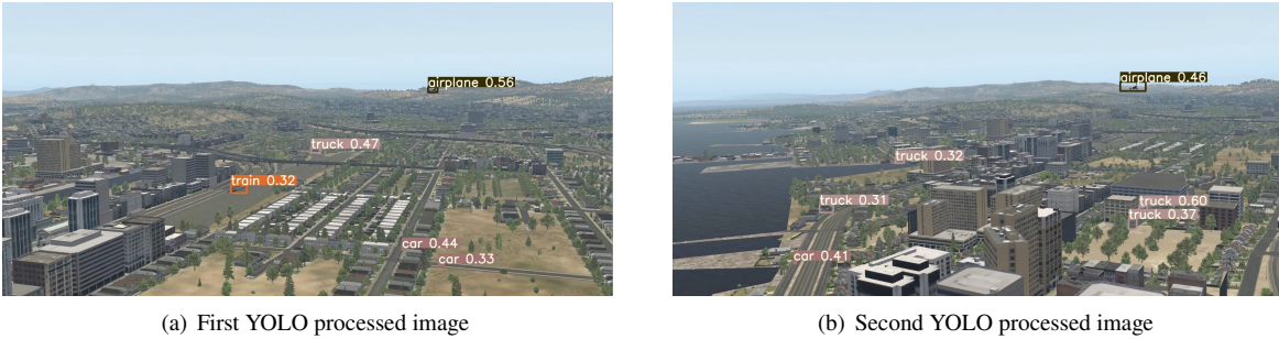
Fig. 4 Two YOLOv3 annotated image examples from x-plane simulations of the aircraft encounter described in Section II. The detection details include the class of the detected object (e.g., “airplane”), the bounding box for the detection, and the confidence level of the detection as a float between 0 and 1.
