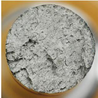
SEM analysis on fracture surface to determine fracture mode, amount and distribution of Cu-rich precipitates
