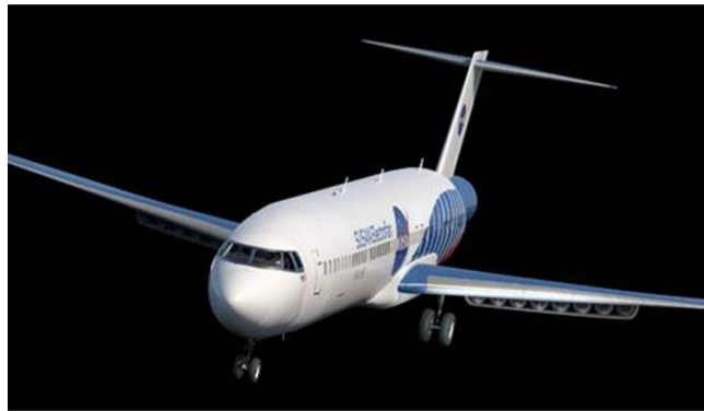
Figure 1: A provisional layout of the turboelectric SUSAN electro-fan aircraft at conceptual design stage.
