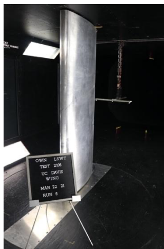
Fig. 9 Downstream view of NLR7301 main element installed in wind tunnel test section.
