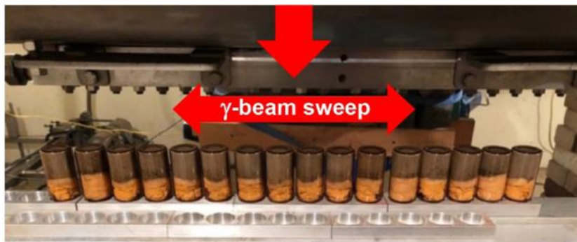
Figure 1 Photo of small vials containing Erbium deuteride fuel radiated by the gamma beam to investigate Lattice Confinement Fusion.
