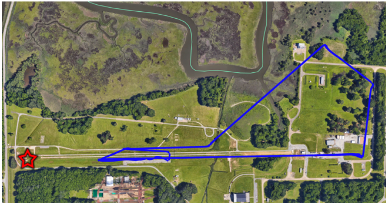
Figure 9: Ground to Air Flight Trajectories superimposed on Google Earth rendered image. Head-on style encounter with the sensor rig shown indicated by the red star and the multirotor by the blue path.
