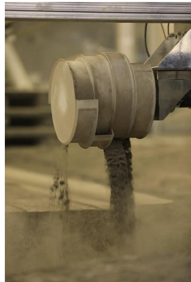
Figure 11. Bucket drum dumping collected regolith
