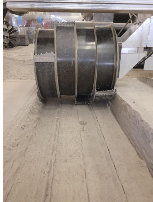
Figure 7. Bucket Drum Test Bed being precision leveled
