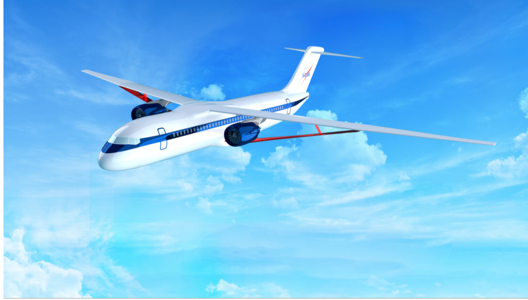
Figure 1 Boeing SUGAR Mach 0.8 Transonic Truss-Braced Wing (TTBW) Aircraft Concept
