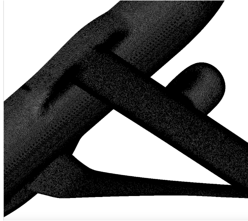
Figure 13 Close View of Mach 0.8 TTBW CFD Mesh
