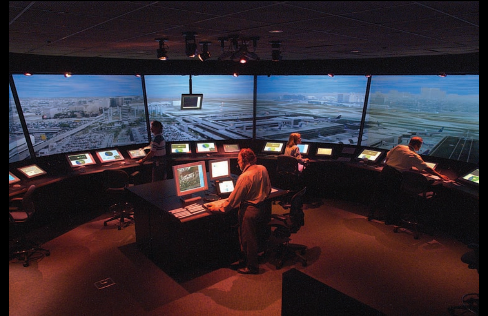
FutureFlight Central simulator interior, configured to recreate the Los Angeles International Airport tower.
