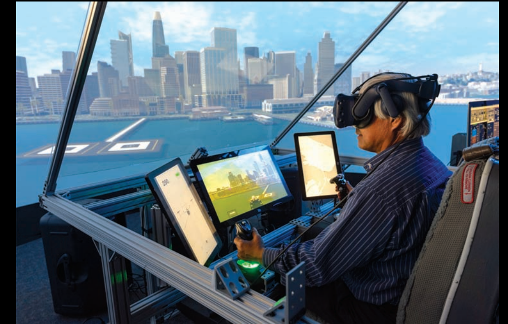
The Aerospace Cognitive Engineering Lab Rapid Automation Test Environment at Ames showing out-the-window views of San Francisco for an Advanced Air Mobility ride quality simulation project.
