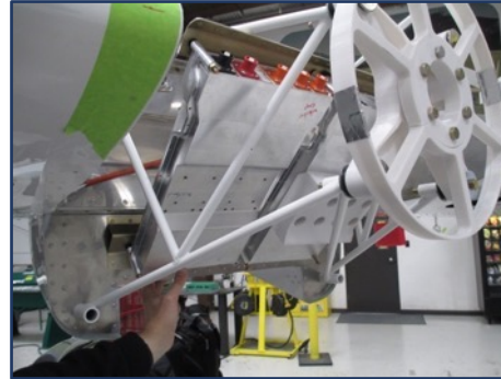
Cruise Motor Mount and Torque Controllers (Inverters)
