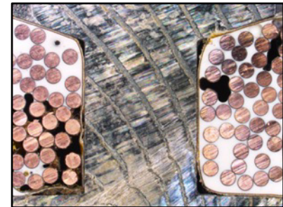
Improved fabrication process still exhibits some voids
