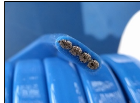
Flat Cable Custom X-57 Design for Electric Propulsion Systems 28
