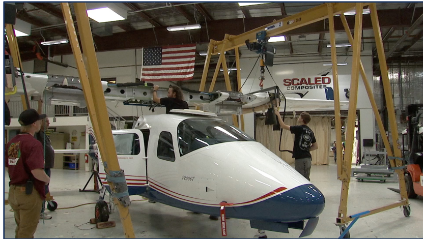
Mod II Wing installation
