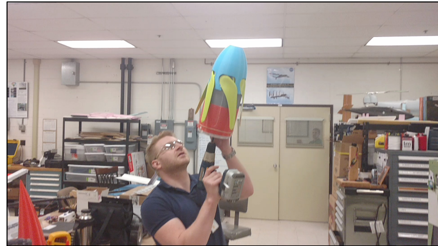
Rapid Prototype 3-d Printed Model of the Initial High Lift Folding Propeller
