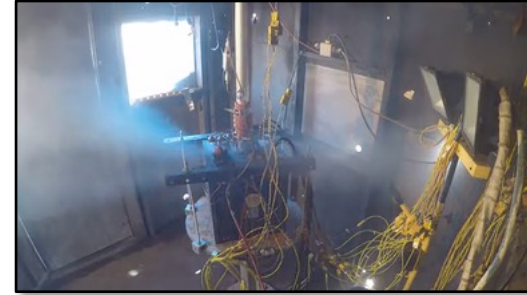
Original battery failed containment propagation test in Dec 2016
