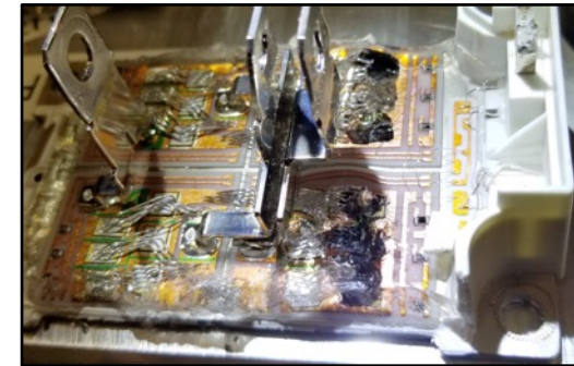
MOSFET body catastrophically failed due to excess current/heat or voltage/vibration (analysis in work)
