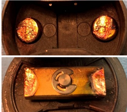
Failed contactor (brazed closed)
