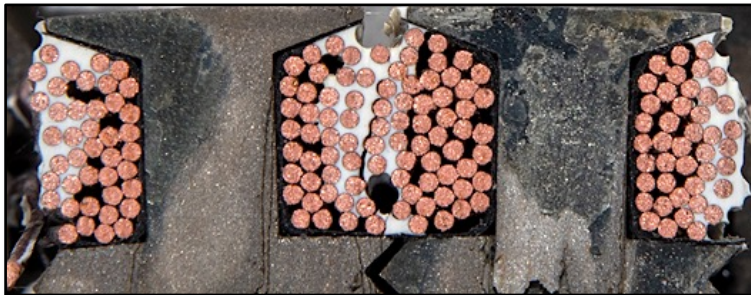
Original motor winding poor epoxy penetration (typical throughout)
