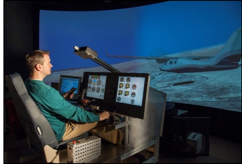
Piloted Simulator at AFRC Includes Flight Like Instrument Panels, Switches, MFD
