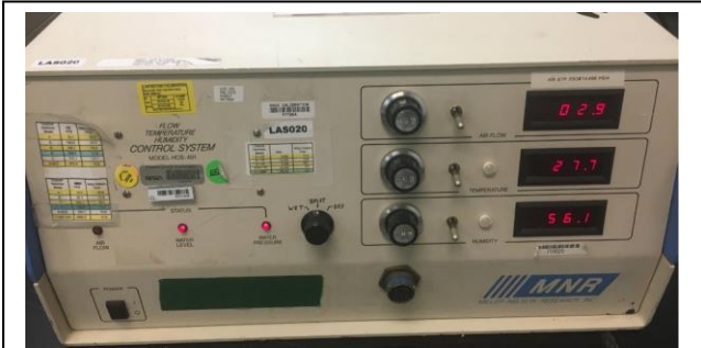
Figure 10. A Miller-Nelson HCS-401 humidifier is used to generate humid gas streams.
