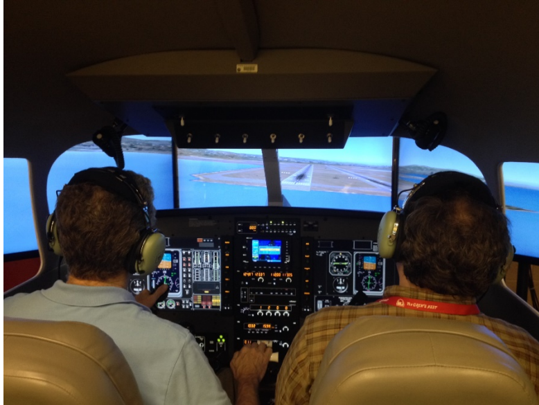
Figure 4.—Interior view of flight simulation test bed for piloted evaluations.
