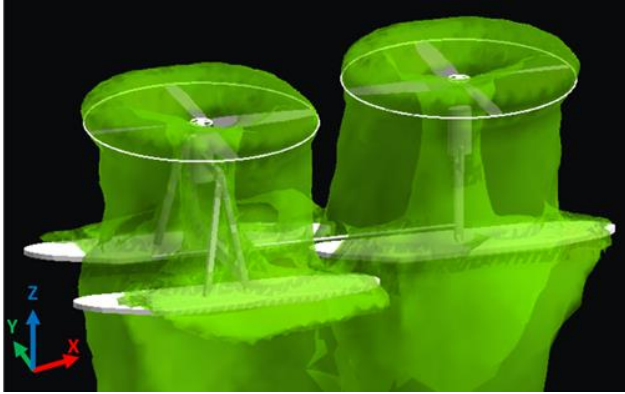
Figure 17. LILI in hover mode: velocity magnitude iso surface flow field prediction ( \theta_{S, front} = 0^\circ , \theta_{0, front} = 10^\circ , C_{T, front} = 0.0253 , \theta_{S, rear} = 0^\circ , \theta_{0, rear} = 10^\circ , C_{T, rear} = 0.0260 ).
