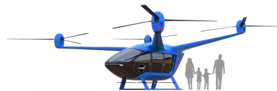
Figure 1a. NASA 6-passenger quadrotor concept vehicle, shown with 3 blades per rotor, Ref. 2.
