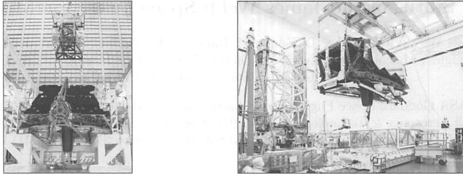
Figure 1: Left: OTIS integration of the science instruments with the telescope at the NASA Goddard's high bay clean room. Right: After environmental testing, OTIS was delivered to NGSS for integration with the Spacecraft Element.
