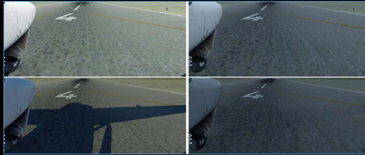
Example input images to a center-line following algorithm, rendered in X-Plane. Left/right = clear/cloudy weather. Top/bottom = 12 pm/4 pm.
