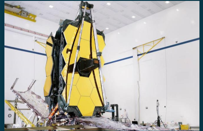
Aug 2019: OTIS is joined to the Sunshield and SCE, completing the assembly of the JWST observatory
