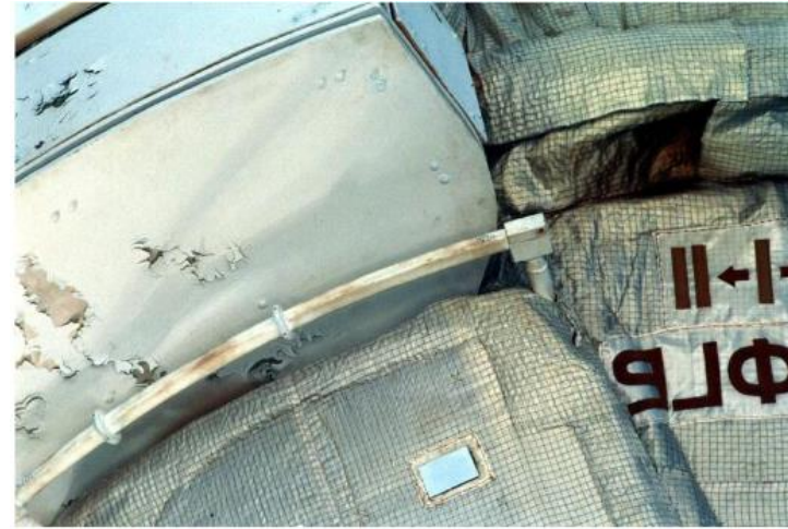
Figure 6: Flaking of the FGB MM/OD shield paint (4A, STS 97-304-001)
