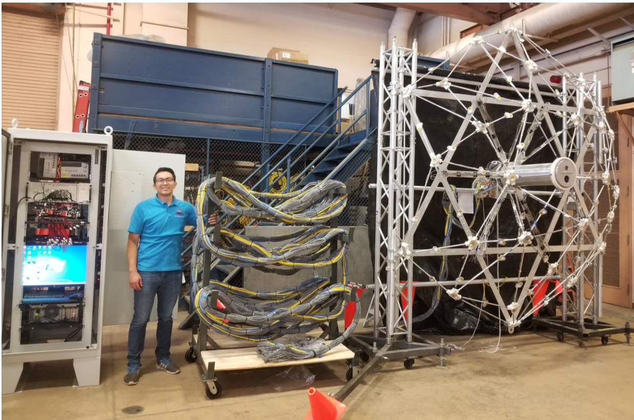
Fig 1. Photograph of the phased array frame, cable bundle and the electronic cabinet.
