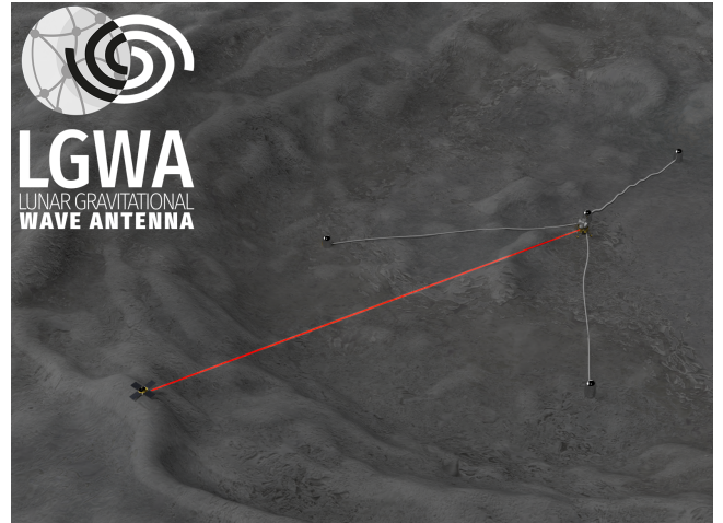
FIG. 2. Star-like deployment configuration of four LGWA stations in a kilometer-scale array equipped with cryogenic inertial sensors. The LGWA deployment site is one of the permanently shadowed regions inside a crater at the lunar north or south pole. A laser-power beaming system is shown as a possible power system for LGWA [11].
