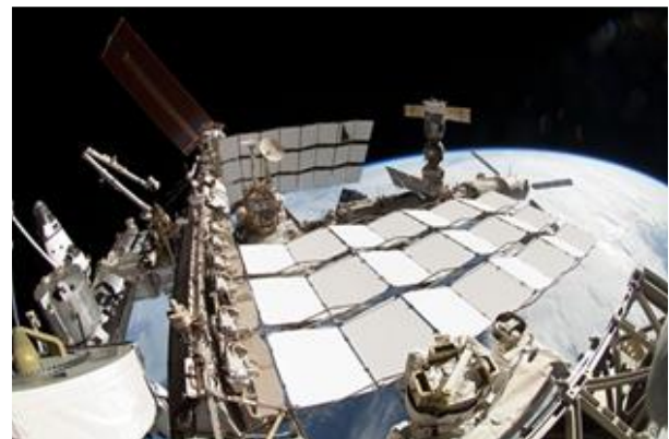
Figure 3. ISS Heat Rejection System Radiators
