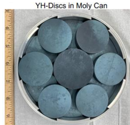
Example yttrium hydride coupons fabricated at Los Alamos
