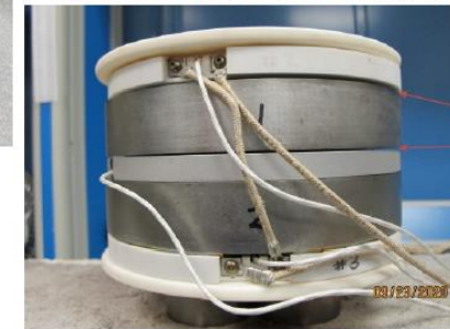
YH-Discs undergoing thermal aging
