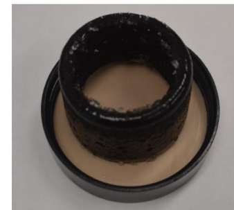
Carbon preform infiltrated with ZrO 2 sol gel (pre-formed annular jacket on inverted jar lid).
