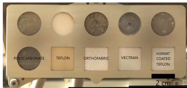
Figure 1: Image taken by the SHERLOC/WATSON camera on the Mars 2020 rover, on Sol 26 of the mission, showing the five space suit materials on Mars. (PDS)
