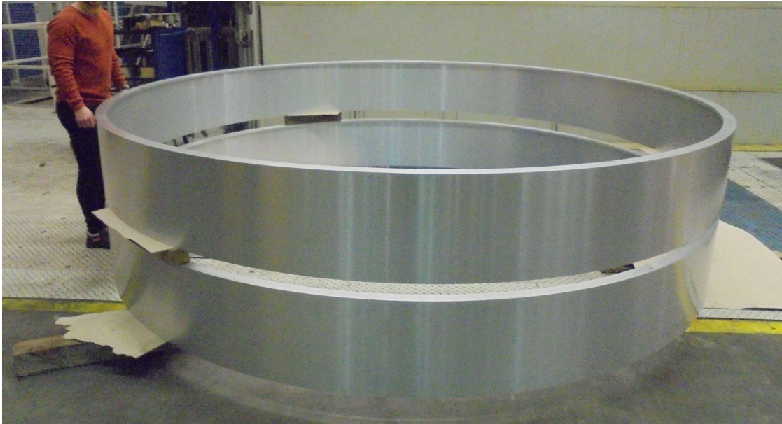
Figure 10. Example of two 10-ft. diameter aluminum ring preforms.
