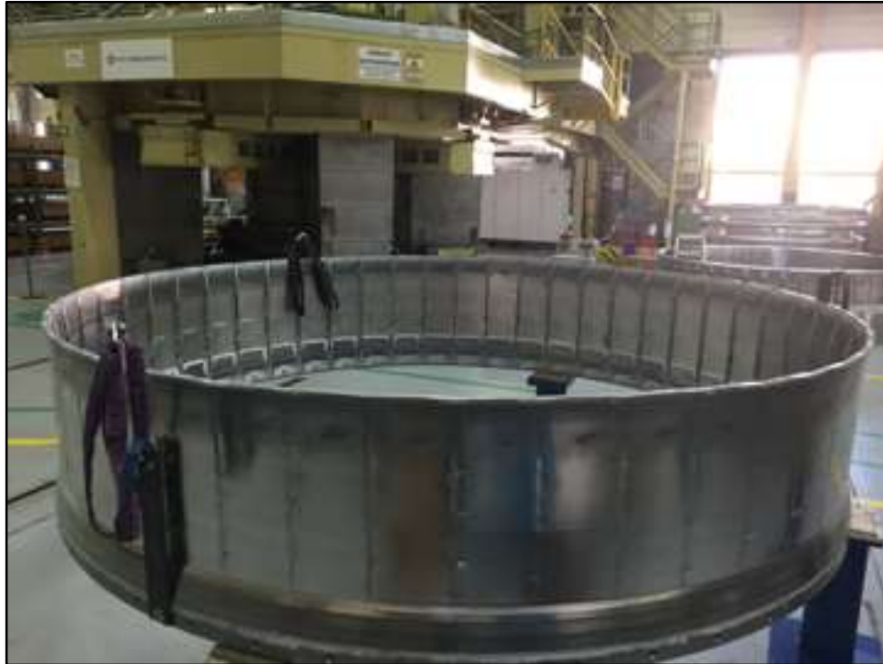
Figure 13. Successfully formed 10-ft. diameter ISC from 2017 forming campaign.
