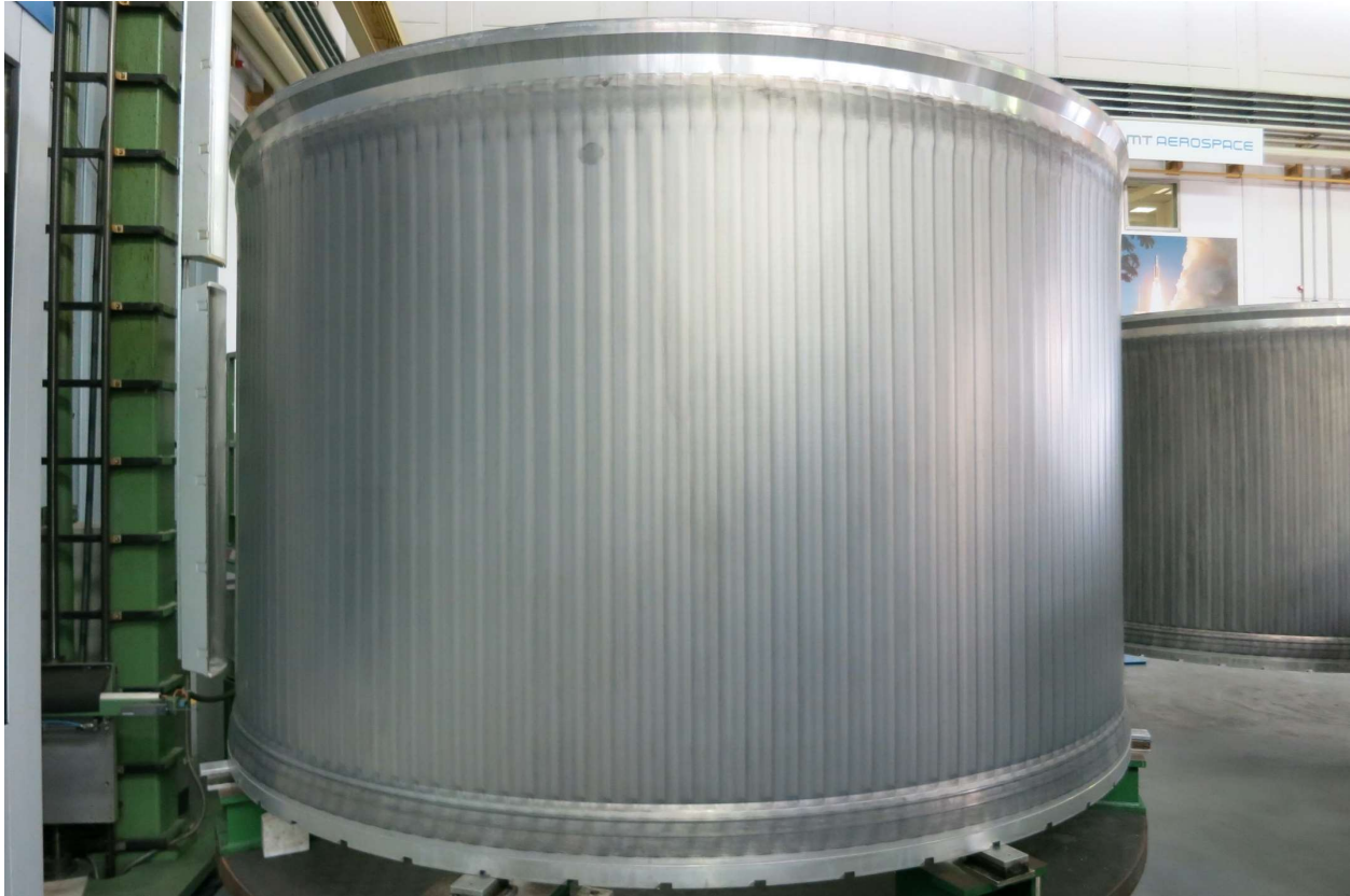
Figure 15. One of four, 10-ft. diameter by 6-ft. long, Al 6061 ISCs formed during the 2020 AATT forming campaign.
