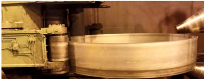
Figure 9. Preform fabrication process at Scot Forge.
