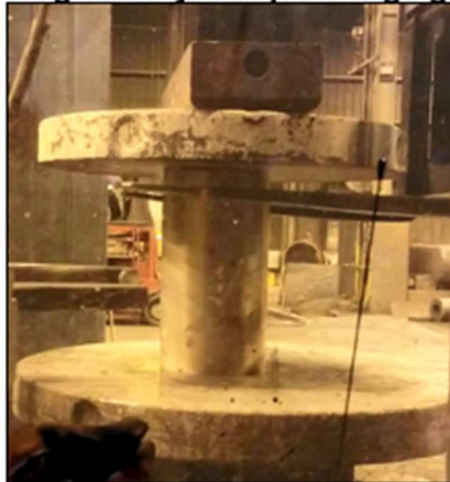
Cross forging to develop desired microstructure
