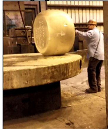
Cross forging to develop desired microstructure
