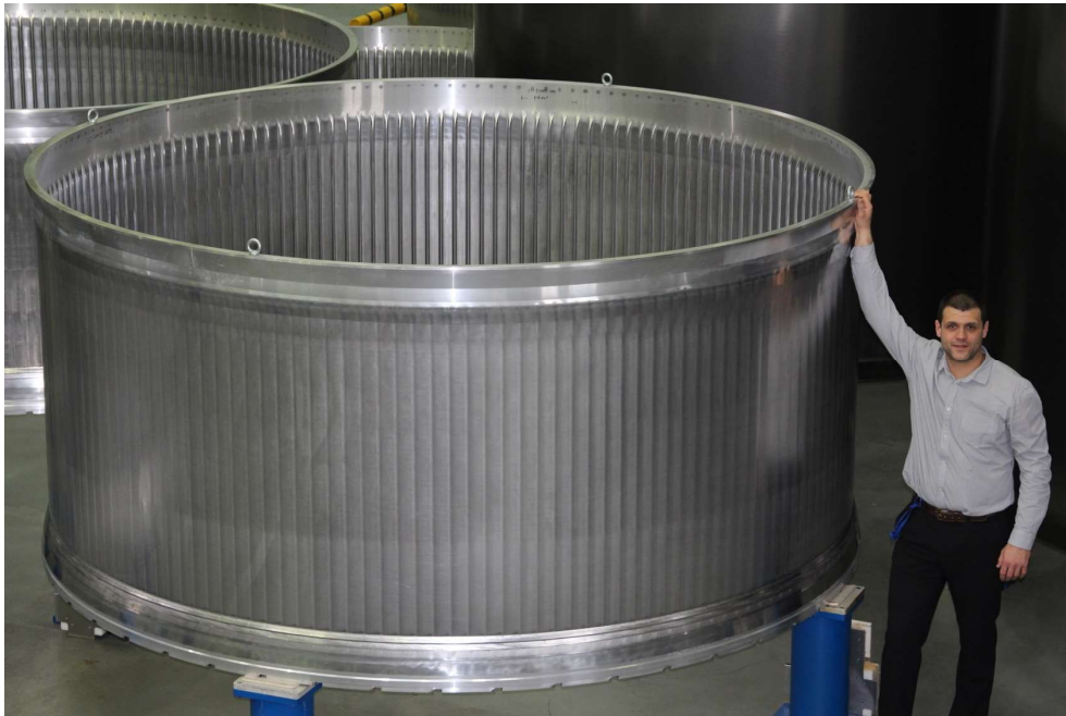
Figure 14. 10-ft. diameter Al 6061 ISC produced in 2019.
