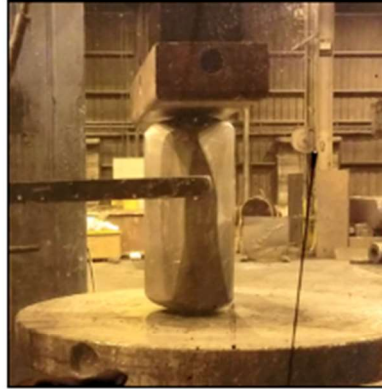
Piercing the ingot and opening the hole
