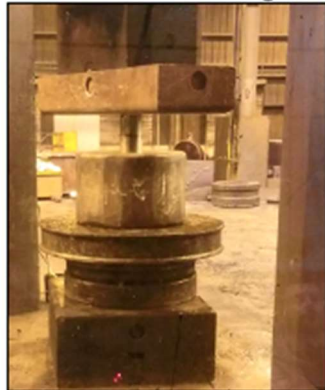
Piercing the ingot and opening the hole
