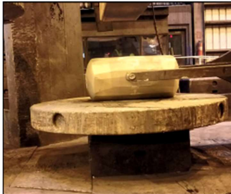
Piercing the ingot and opening the hole
