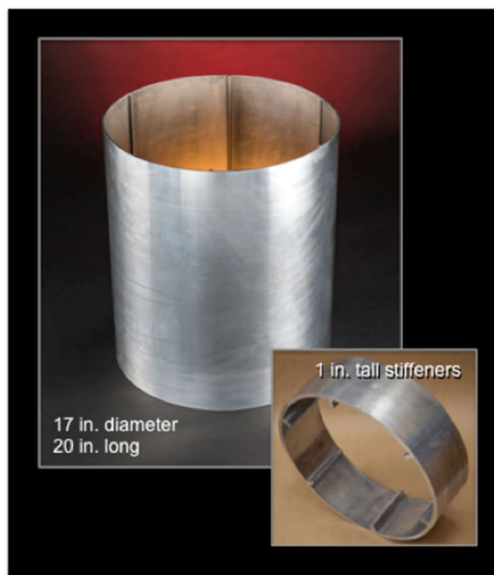
Figure 8. Sounding rocket scale cylinders – as-formed sounding rocket cylinder (top) and segment from a 17-inch diameter cylinder with 1-inch tall stiffeners (inset).
