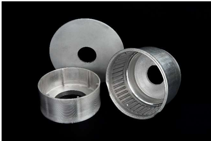
Figure 7. Subscale, 8-inch diameter clutch housing (right), ISC (left) and preform disk (rear).
