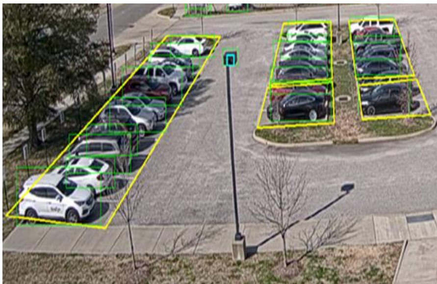
Figure5. LaRC Park: R-CNN parking lot occupancy detection at NASA Langley
