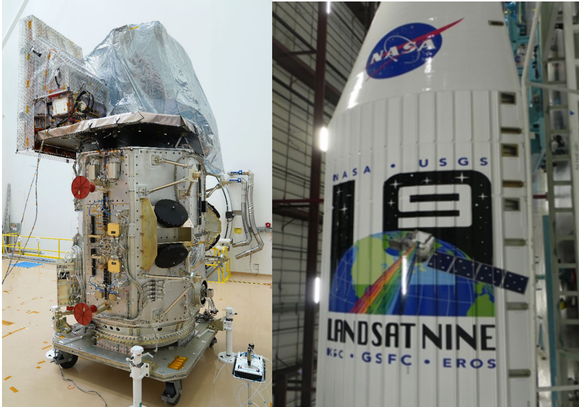
Figure 2. Landsat 9 observatory with integrated OLI-2 and TIRS-2 instruments (bagged) (left) and Atlas-V payload fairing for Landsat 9 (United Launch Alliance Photo) (right).
