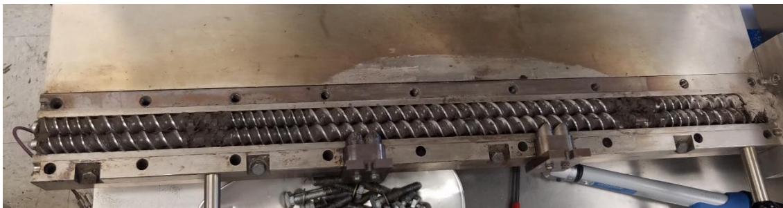
Figure 20. The twin screw extruder in an opened configuration directly after testing.
