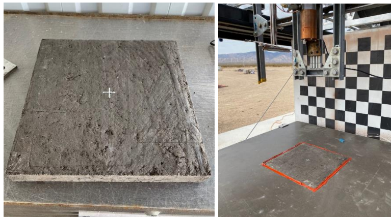
Figure 5. 11% RTV-Regolith paver before (left) and after installation on the test stand (right).
