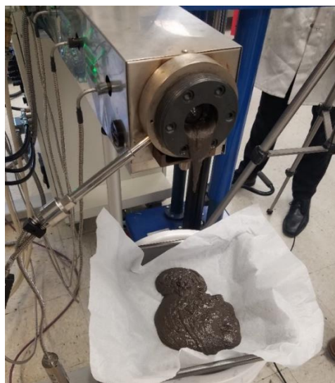
Figure 12. 80/20 wt% BP-1/RTV material exits the extruder.
