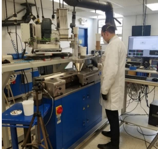
Figure 15. The twin screw extruder is configured prior to testing.
