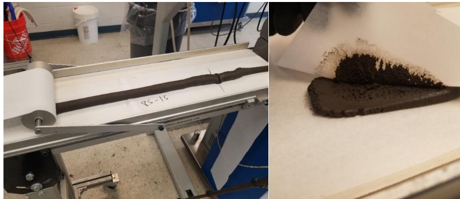
Figure 18. A roller attachment is installed on the conveyor to compact the materials after deposition(left). Materials stick to the parchment paper after they have been compressed (right).
