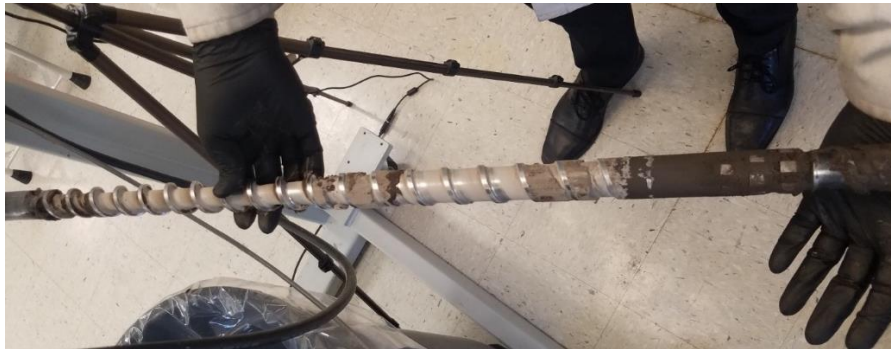
Figure 146. The extruder screw has inconsistent residual materials along its length.
