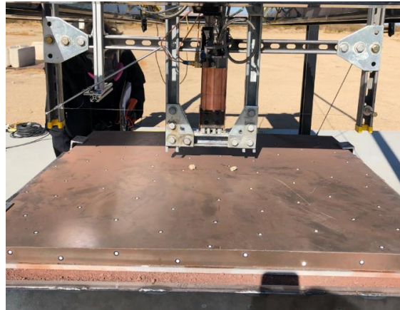
Figure 4. 20% RTV-Regolith paver installed on the test stand prior to testing.
