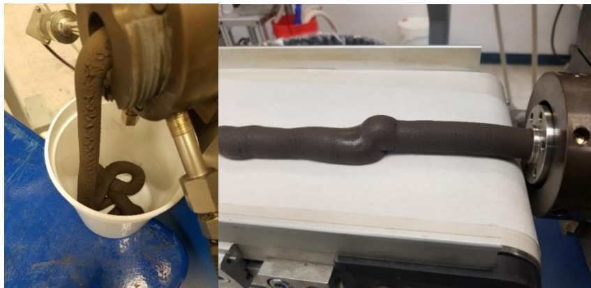
Figure 16. Extrusion of 85/15 wt% BP-1/RTV without the die (left) and with the die (right).
