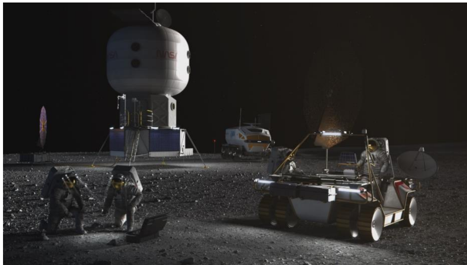
Figure 2: An artist's concept of the Artemis Base Camp with the three proposed primary mission elements – the Lunar Terrain Vehicle (unpressurized rover), the Pressurized Rover, and the Surface Habitat
