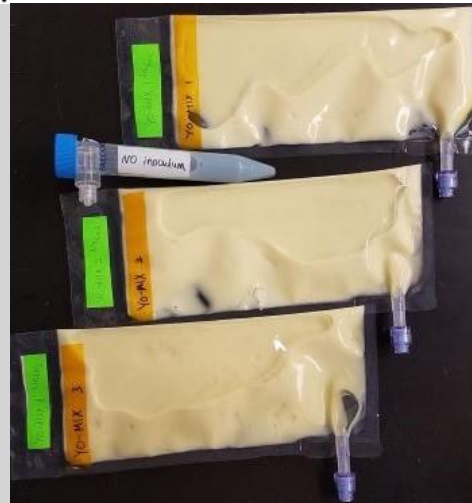
BN-1 hardshell bioreactor growing yeast expressing carotenoids in SABL on the ISS. BN-2 FEP bag growing yogurt with a pH indicator dye on during pre-flight testing
