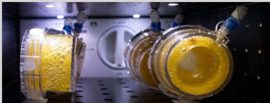
BN-1 hardshell bioreactor growing yeast expressing carotenoids in SABL on the ISS. BN-2 FEP bag growing yogurt with a pH indicator dye on during pre-flight testing
