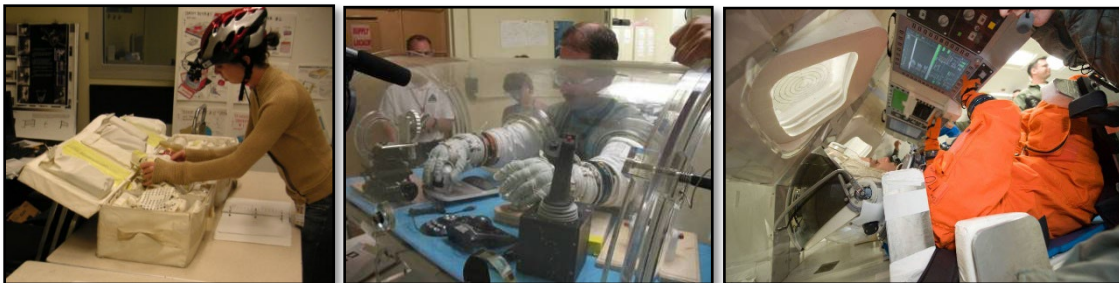
Figure 1. Examples of HITL evaluations from ISS Program (left, medical kit design evaluation) and Orion Program (center, glove-box evaluation of hand controller designs for use with pressurized gloves; and right, micro-gravity parabolic flight evaluation of display and control layout, window field of view, and seat design).
