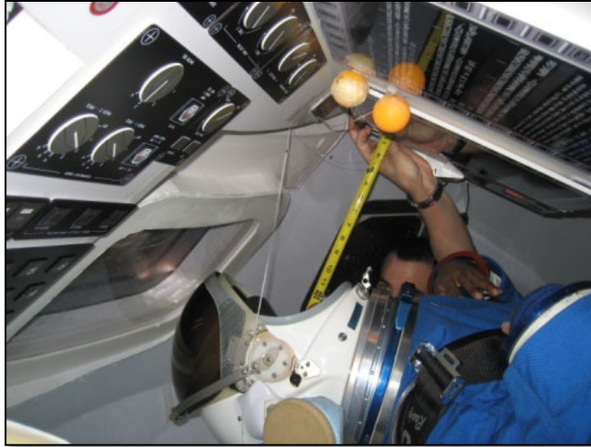
Figure 3. Example of a low-fi mockup of the Orion capsule being used to evaluate design eye-point, viewability, and reach related to seat design, location, display and control panel layout, and launch-entry-ascent suit design impacts.
