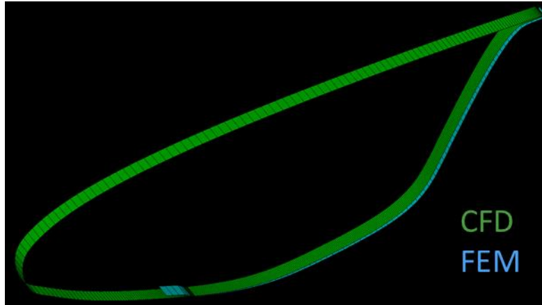
Figure 4-26. CFD mesh conversion results in CFD and FEM overlay.
