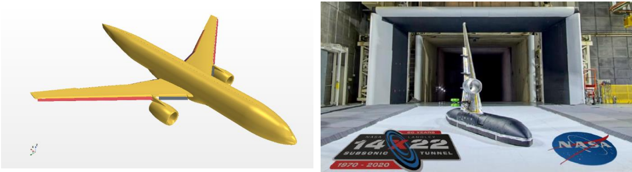
Figure 2-1. CAD representation of baseline CRM-HL geometry (left) and half-symmetry model testing in NASA LaRC 14×22 tunnel (right, from Lockard et al. [22]).
