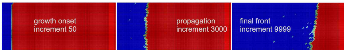
(g). DEBONDING FORCE=RAMP, unstable growth tolerance, nonlocal, \alpha=0.9 , \beta=1E10 , n=1 ( \Delta B=0.5 mm).
