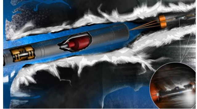
Fig. 1. Artistic rendering of a robotic probe (i.e., Europa Tunnelbot) capable of melting and/or drilling through icy crusts of planets, moons, or asteroids 3 .
