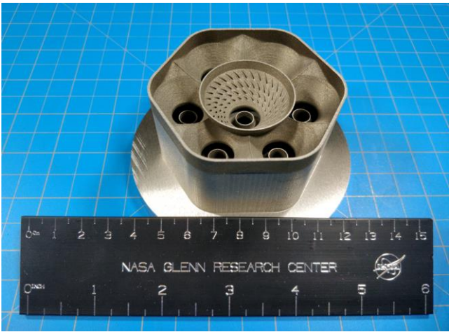
3D Printed ODS Combustor Dome
