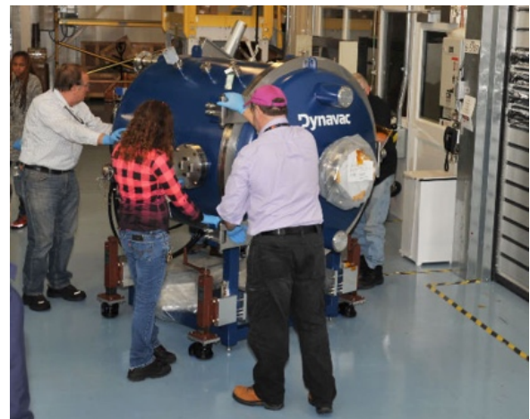
Figure 2-7. Optical Module Level TVAC Test Set-up
