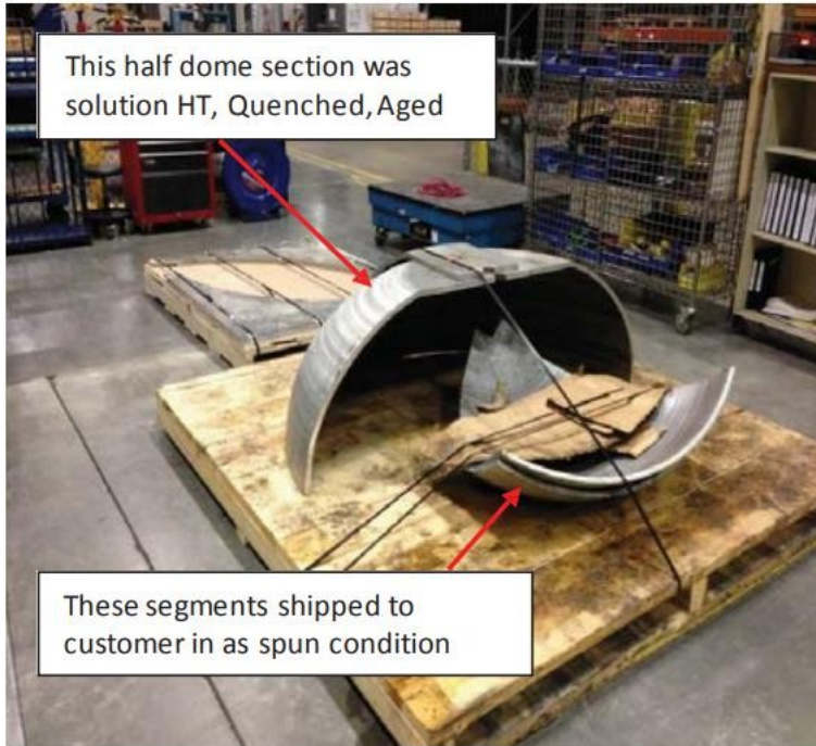
2014 NASA Report on 0.75" thick 2195 FSW SF Dome
