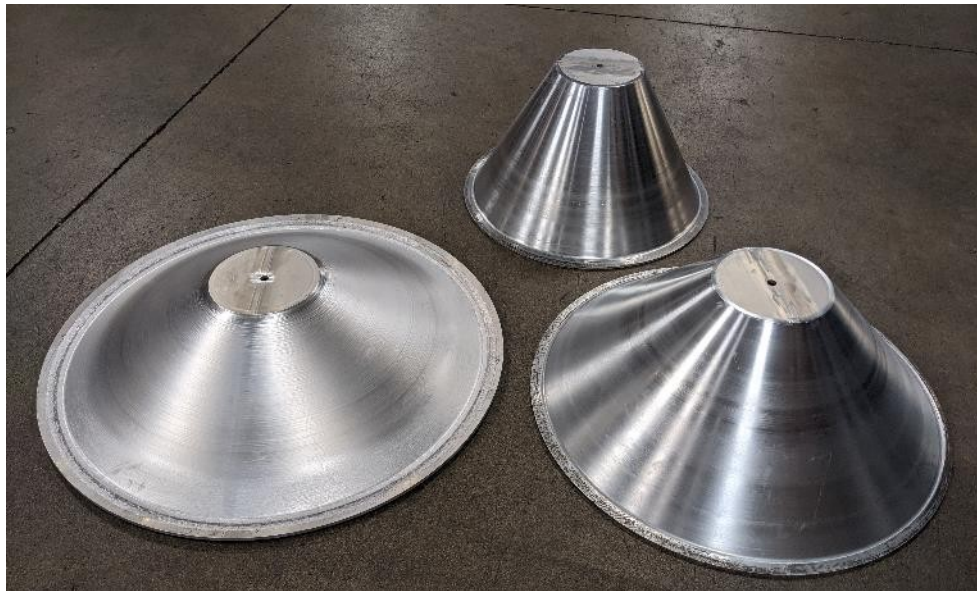
Waterjet Cutting (Post-Weld Heat Treating) Tooling Setup Spin Forming Post-Spin Form Heat Treating
