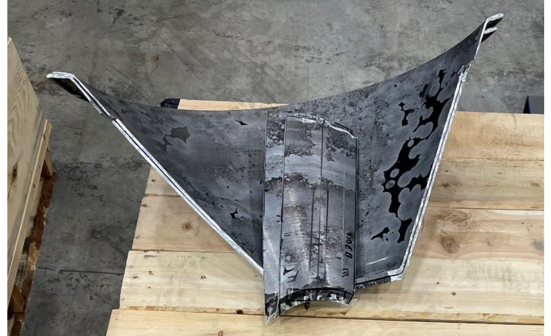
Current Work 0.32" thick 2050 FSW SF Dome (30° Strain)
