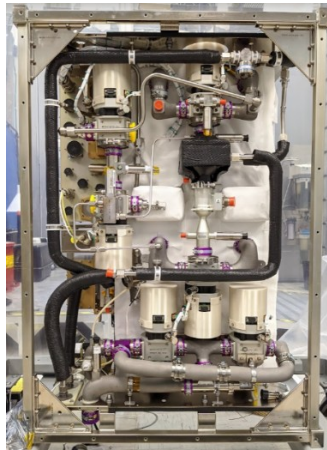
Figure 2. Four Bed CO 2 Scrubber Flight Hardware.
