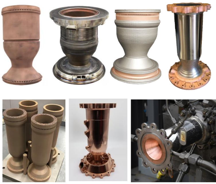
Laser Powder Bed Fusion (L-PBF) Copper Alloys combined with other AM processes to provide bimetallic
