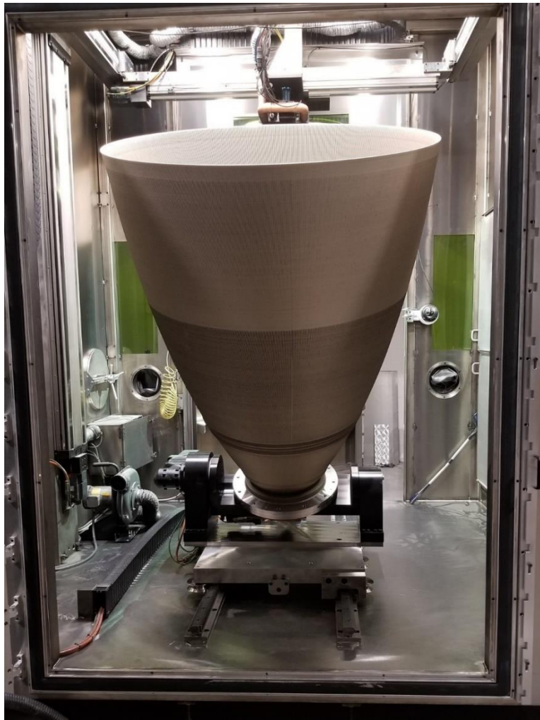
60" (1.52 m) diameter and 70" (1.78 m) height with integral channels 90 day deposition
