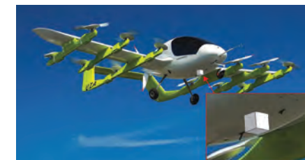
Concept for a ubiquitous weather sensing pod for advanced air mobility vehicles. A sensor pod and the vehicle itself potentially could be used to collect atmospheric measurements during flight.
