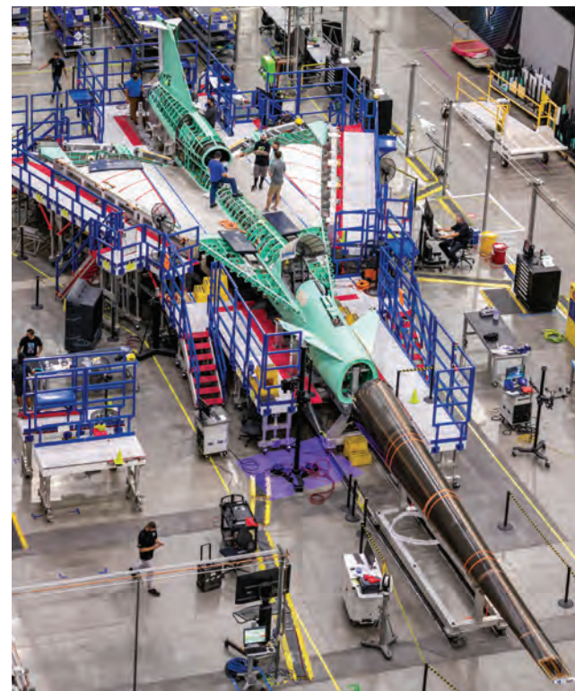
Construction and assembly of the supersonic X-59 QueSST research plane at Lockheed Martin Aeronautics Company's Skunk Works® factory Credit: Lockheed Martin
