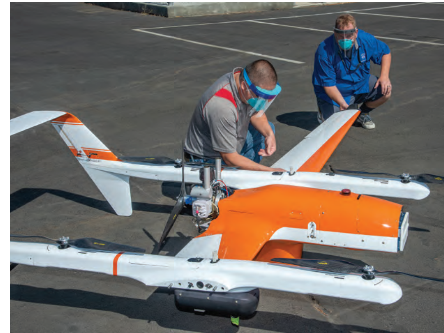
The Resilient Autonomy project team conducted basic functional flight tests of the EVAA-modified HQ-90, a vertical lift and transition remotely piloted aircraft.
