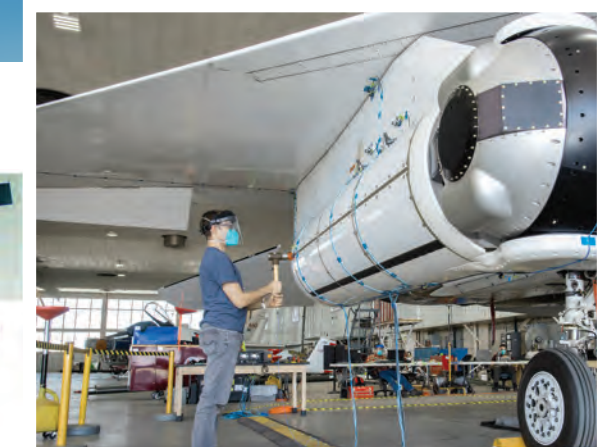
(Above) F-15D TN 897 with new wing store (STA 2) during a compatibility flight profile flight in 2020; (below) GVT and FEM mode shape comparisons of F-15 wing pylon and new wing store; and (right) lateral impact hammer excitation on wing store during GVT
