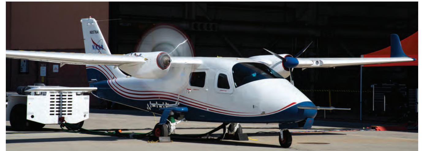
The X-57 aircraft undergoes high-voltage ground testing. Principle goals of the X-57 project are to share the design and airworthiness process with regulatory and standards organizations and establish the aircraft as a reference platform.
