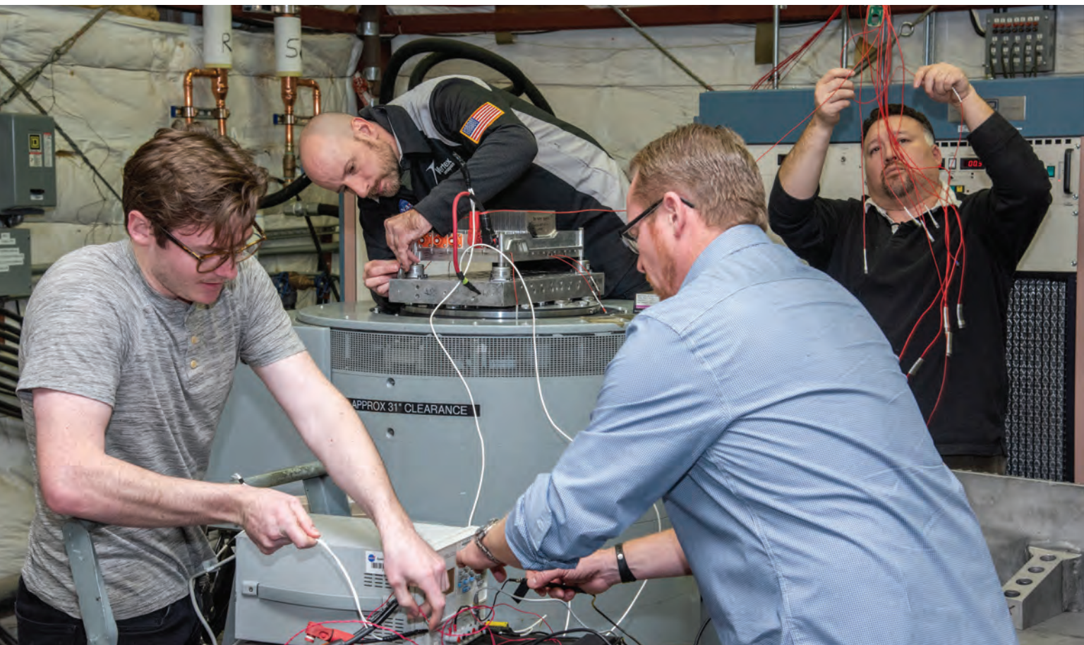
Engineers from NASA Armstrong and Empirical Systems Aerospace prepare a cruise motor controller for use on the all-electric X-57 aircraft for vibration testing.
