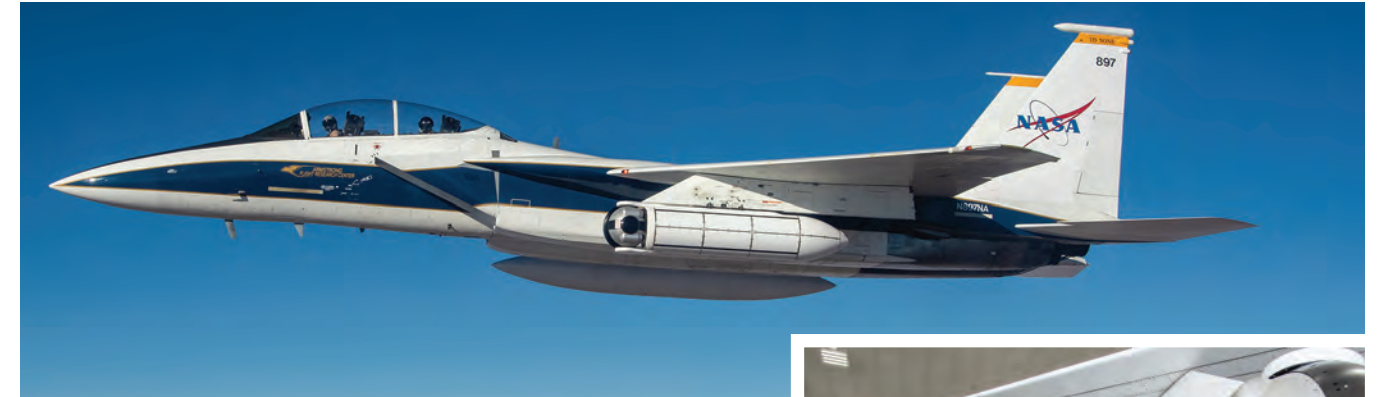
(Above) F-15D TN 897 with new wing store (STA 2) during a compatibility flight profile flight in 2020; (below) GVT and FEM mode shape comparisons of F-15 wing pylon and new wing store; and (right) lateral impact hammer excitation on wing store during GVT
