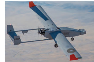
The Navmar Applied Sciences Corporation TigerShark aircraft flew over Edwards Air Force Base in July 2019 during a series of flight tests to support development of DAA standards for medium-sized UAS.
