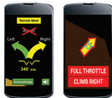
NASA Armstrong's iGCAS can be used for a variety of aircraft, including general aviation, helicopters, and unmanned aircraft. The technology has been incorporated into an application for tablets and other handheld/mobile devices.
