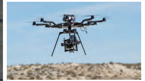
The Resilient Autonomy project team conducted basic functional flight tests of the EVAA-modified HQ-90, a vertical lift and transition remotely piloted aircraft.
