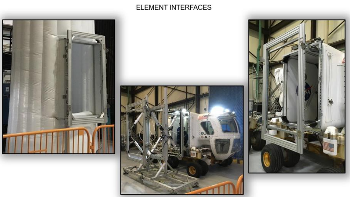
Fig. 10.2-6: Proof of concept for surface docking and pressurized transfer hardware under development at NASA intended to feed most notional lunar surface architectural roadmaps and near-term development activities for future commercial development and deployment.
