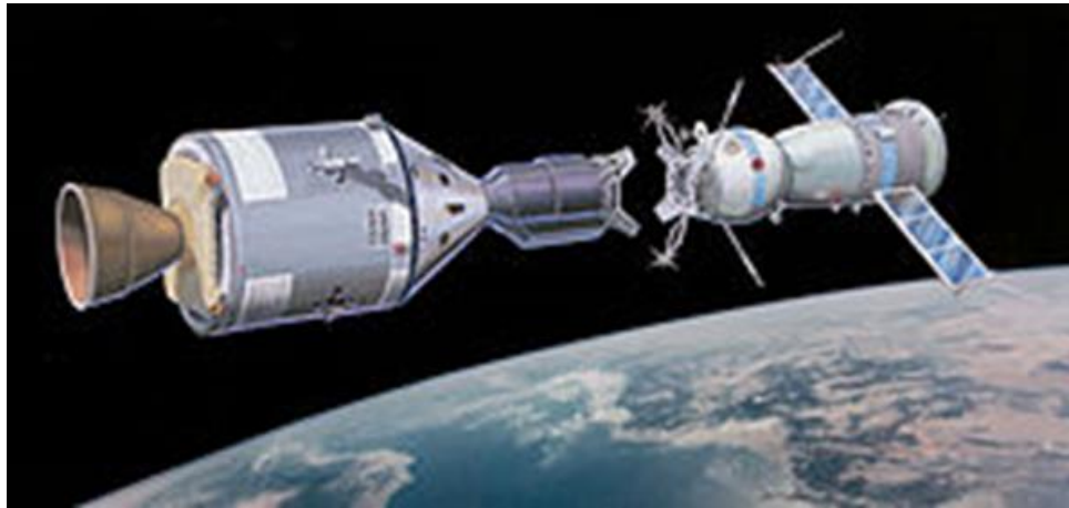
Fig. 10.2-1: Artist's conception of the Apollo and Soyuz docking using the 3-petal androgynous mechanism (Credit: NASA)
