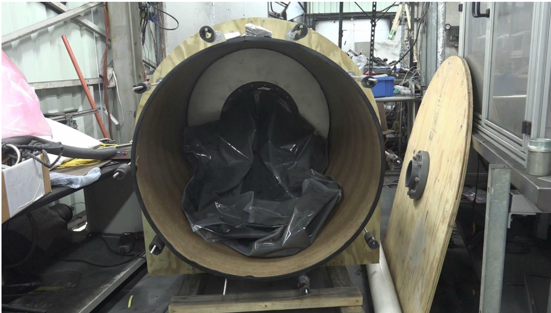
Gas Collection System Test (End Cap Removed)
