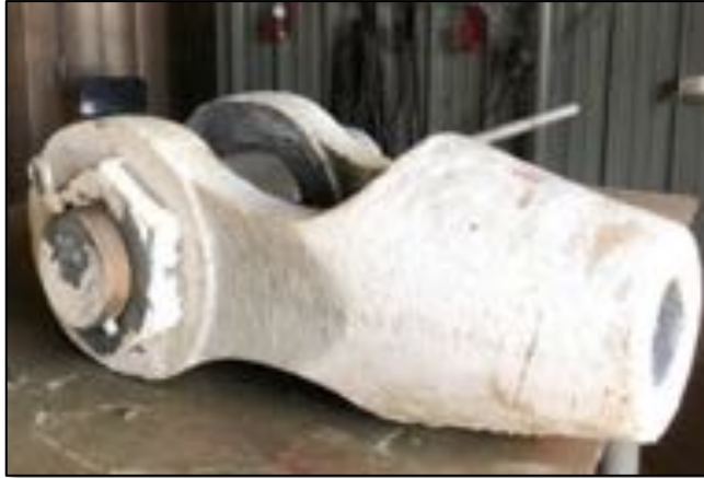
Aux M4N Failed Socket
