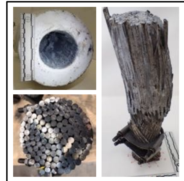
Comparison of forensics (left) with modeling predictions just prior to failure (center/right)
