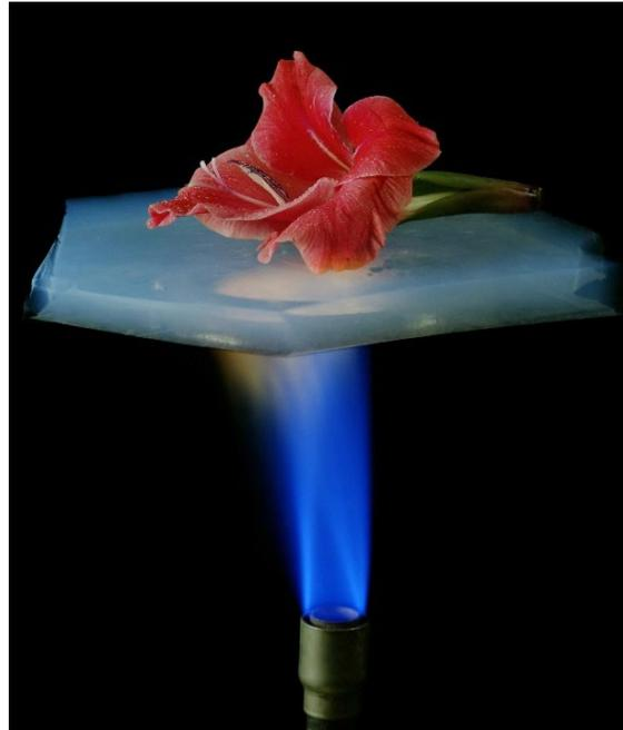
Highly porous structure of aerogel is responsible for its extremely low thermal conductivity.
