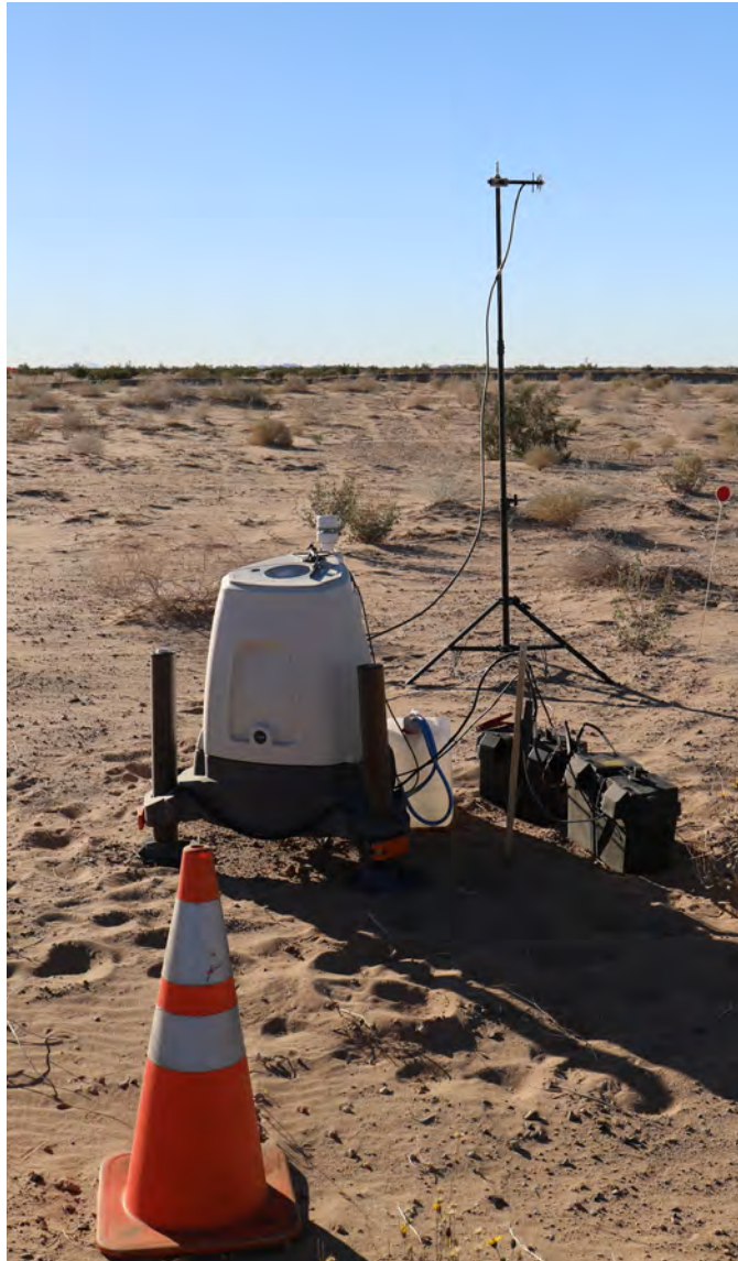
Figure 11: LIDAR, as deployed.
