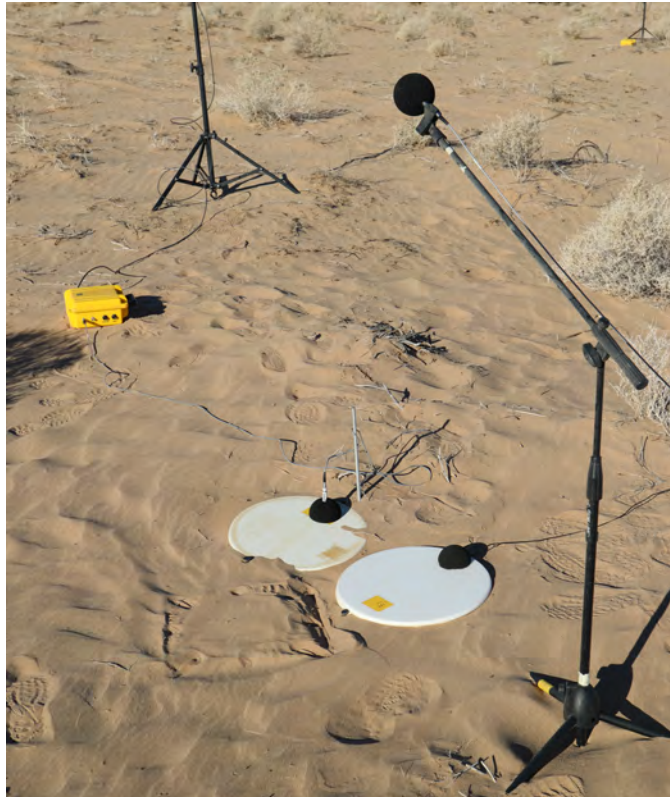
Figure 5: Tri-located microphone setup for microphones 31 (GRAS 67AX), 64 (B&K 4189 inverted), and 65 (B&K 4964 on 4 foot tripod).
