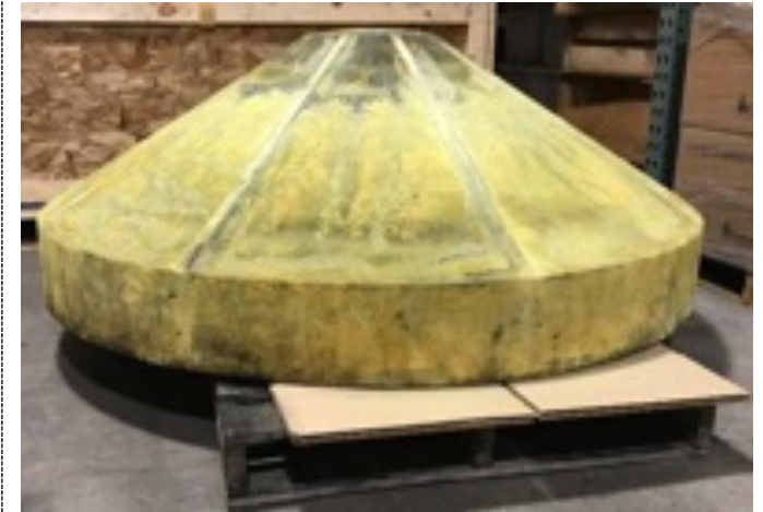
Extended single piece heatshield manufacturing demonstrated recently
