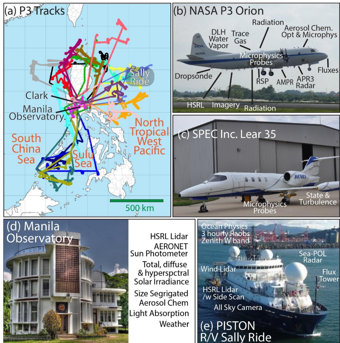
Figure 3. Flight tracks and instrumentation. (a) Flight tracks for 19 NASA P-3 flights conducted between Aug 25-Oct 5, 2019. Also noted is the Clark airborne base of operations and the operations area of PISTON's R/V Sally Ride collection; (b), (c), (d), and (e) Key P-3, SPEC Learjet 35, Manila Observatory and R/V Sally Ride instrumentation. AERONET=Aerosol Robotic Network; AMPR=Advanced Microwave Precipitation Radiometer; APR3=Airborne Precipitation Radar 3 rd generation; DLH= Diode Laser Hygrometer; HSRL=High Spectral Resolution Lidar; RSP= Research Scanning Polarimeter.
